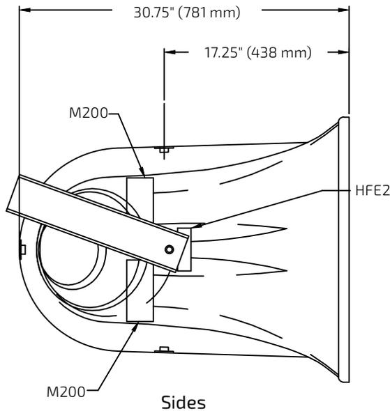
*Note: Cabinets are hand-laminated and measurements vary slightly due to the thickness of the fiberglass. Dimensions shown should not be used to fabricate hanging fixtures. Mounting points are approximate.*
